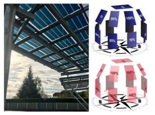
**Figure 2.** *Left* : OPVs in a 2.8 kW<sub>p</sub> grid-connected OPVIUS installation in Pontiacq, France. *Right* : Alignment effects in Si-panels (blue) and in OSCs (red).
